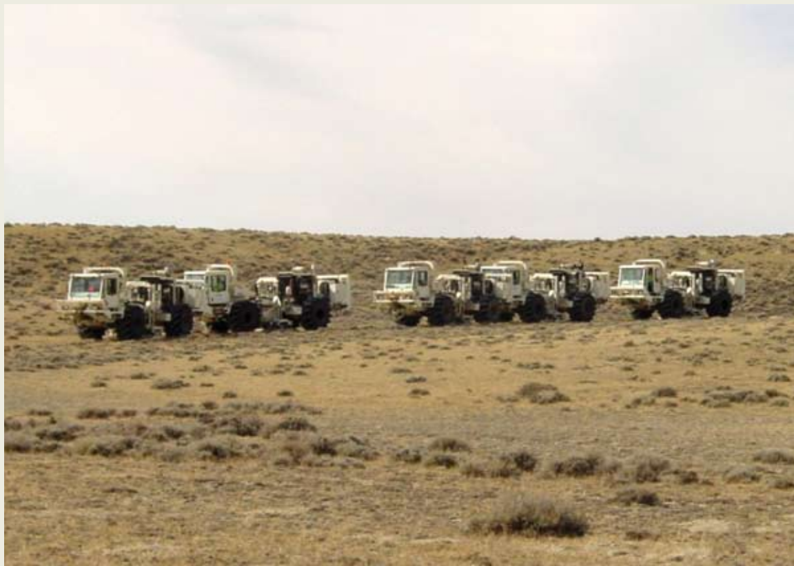
Articulated vibroseis trucks are one of many geophysical exploration methods.
